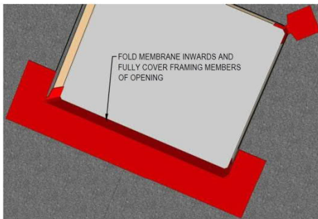
D - FOLD MEMBRANE INTO OPENING
