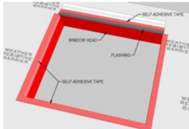
I - INSTALL A SELF-ADHESIVE TAPE ALONG THE EDGES OF THE WEATHER-RESISTIVE BARRIER
